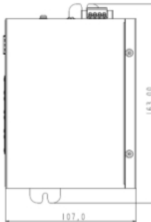
Figure 3 — The switch with the attached wall mounting brackets
