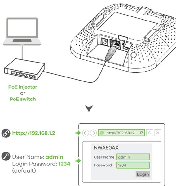
**EN** **1-b** Use an Ethernet cable to connect your computer to the **UPLINK** port of the NWA50AX through a PoE injector or PoE switch. Use its DHCP-assigned IP or default static IP address "http://192.168.1.2" to access the web configurator. Make sure your computer IP address is in the same subnet as the NWA50AX's.
