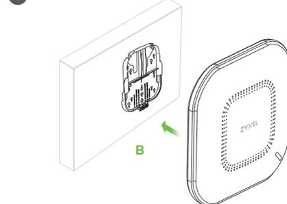
**EN** **2** Install two mounting screws through the holes on the bracket (B) into the plugs/anchors to secure the bracket to the wall/ceiling. Make sure the screws are snugly and securely fastened to the wall/ceiling.
