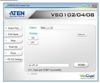
The Switch Port page is used to connect the Video/Audio source to the display ports, and to power on/off displays.
