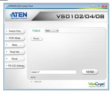
The Reset page is used to reset the VS0102 / VS0104 / VS0108 back to the factory default settings. On the Reset page, the following actions are possible:
