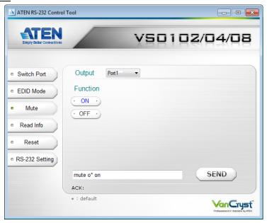
The Mute page is used to turn audio on or off for an output port. On the Mute page, the following actions are possible:
