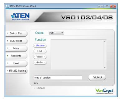
The Read Info page is used to get configuration information from the VS0102 / VS0104 / VS0108, which is displayed in the large text box on the center of the page. On the Read Info page, the following actions are possible:
