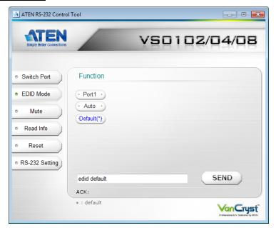
The EDID Mode page is used to set the EDID setting for all displays. The EDID Mode page provides three options - Port1, Auto, and Default(\*), as described below.
