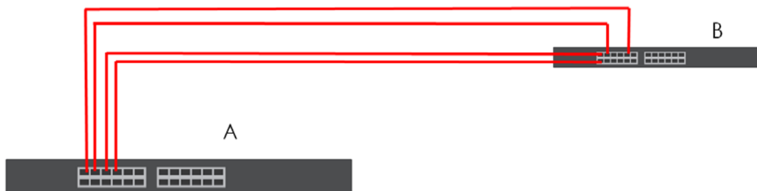
Figure 156 Trunking Example - Physical Connections
