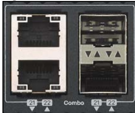
Figure 15 Combo Port Example: 10 Gigabit Port and SFP+ Transceiver Slot
